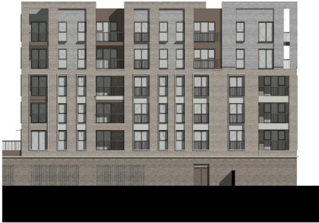
Block E Elevation South-East 1:100
